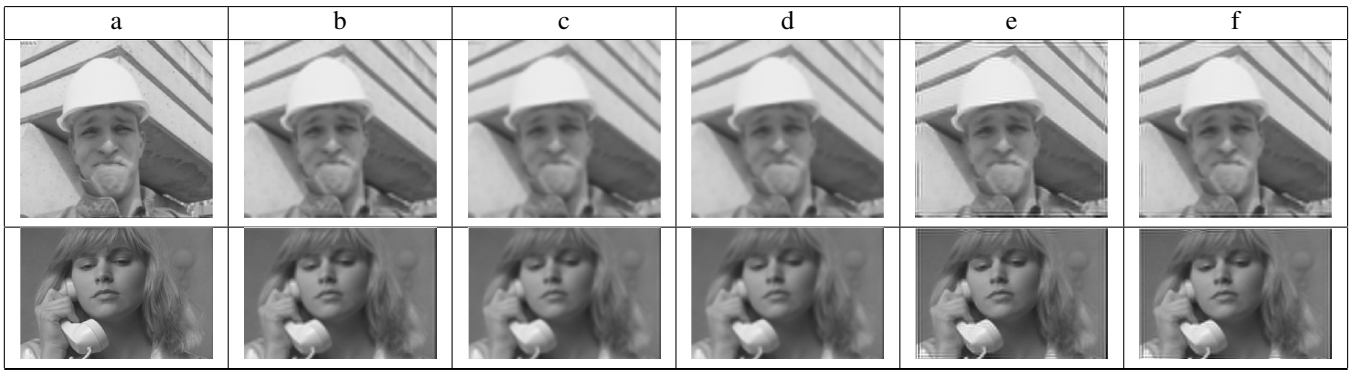
Fig. 4. Benchmark video sequences results. a is the reference image, b is interpolated (bicubic) image, c is the super-resolved image with probabilistic fusion, d is the super-resolved registered into the interpolated one, e is the result of SR after deblurring, and f is the results of alpha-blending of e and b.
