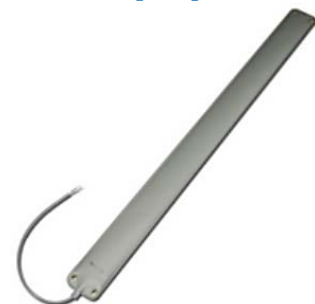
Figure 19 Bed occupancy sensor [282]
