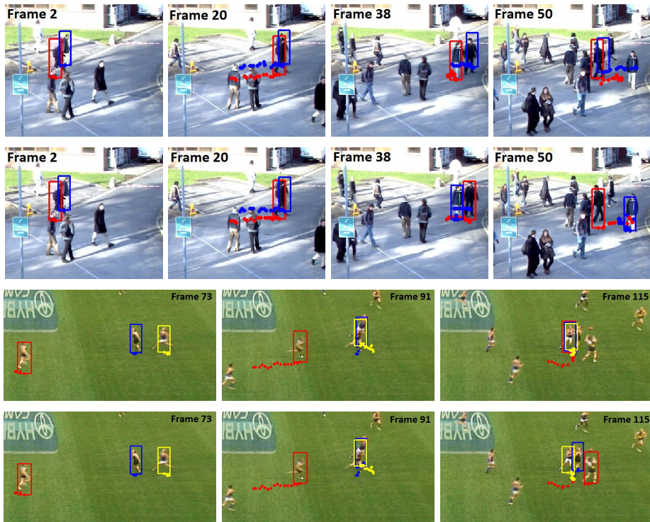
Fig. 3. Visual trackers without (1 st and 3 rd rows) and with (2 nd and 4 th rows) local data association. See text for details.
