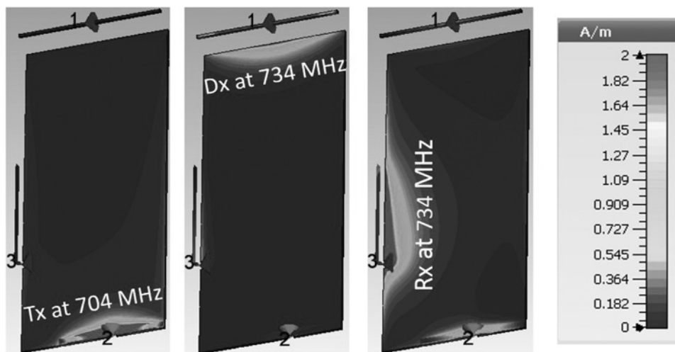
Fig. 12 Current distribution: Tx antenna at 704 MHz, Dx and Rx antennas at 734 MHz
