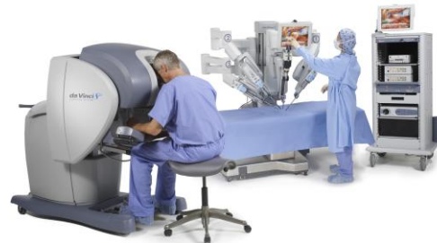
Figure 2: Telesurgery system for one surgeon (left). An assistant (right) is able to see the endoscopic view and draw lines on a touchscreen to visually communicate with the surgeon. ©2014 Intuitive Surgical, Inc.
