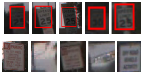
Figure 16. Examples of troublesome US speed limit signs. First row shows missed signs and second row shows false positives.
