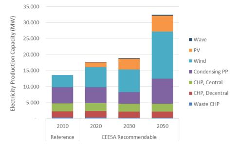
Figure 24: Electricity production capacity in Denmark between 2010 and 2050 for the CEESA Recommendable 100% renewable energy scenario.
