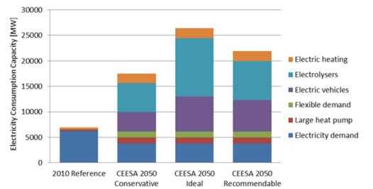
Figure 27: Electricity consumption capacity in Denmark between 2010 and 2050 for the CEESA Recommendable 100% renewable energy scenario.
