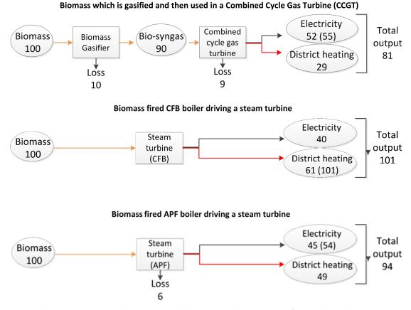
Figure 30: Using biomass in a steam and gas turbine with the potential characteristics of 2050. Values in brackets are assuming operation in bypass mode for the CFB boiler and steam turbine or condensing mode power production for the combined cycle gas turbine.
