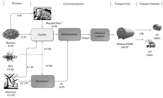
Figure 35: Steam gasification of biomass which is subsequently hydrogenated. <sup>1</sup>The electrolyser efficiency is assumed to be 73% for the steam electrolysis [9,66]. <sup>2</sup>A loss of 5% was applied to the fuel produced to account for losses in the chemical synthesis and fuel storage. <sup>3</sup>Marginal efficiency is assumed to be 125% and the steam share 13% relative to the biomass input.
