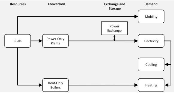
Figure 19: Interaction between sectors and technologies in the Danish energy system until the 1970s.
