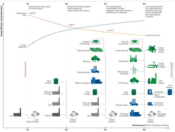
Figure 31: Development of district heating in the past (1<sup>st</sup> and 2<sup>nd</sup> Generation), current district heating technology (3<sup>rd</sup> Generation), and the future of district heating (4<sup>th</sup> Generation) [53].
