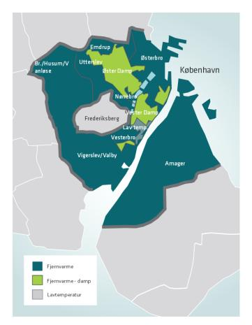
Figure 14: Map of district heating areas in the City of Copenhagen (*Fjernvarme*: District heating, *Damp*: Steam, *Lavtemperatur*: Low temperature) [36].
