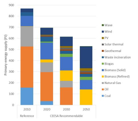
Figure 2: The primary energy supply for Denmark in 2010, in the CEESA Recommendable scenario.
