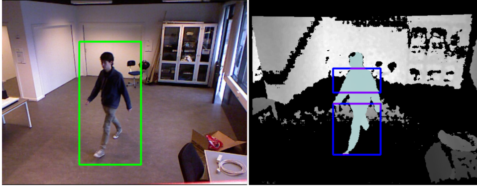
Figure 3: The left image illustrates a detection. On the right, the person has been segmented in the depth image, and the blue boxes illustrates the boxes which are used as basis for the color histograms.
