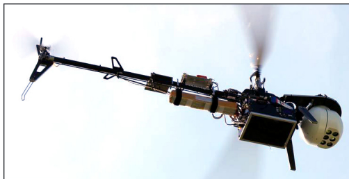
Fig. B.2: The UAS, based on a Maxi Joker 3 RC-helicopter, equipped with a multi spectral camera mounted in a gimbal device (front), a mini-ITX computer (underside), and IMU and GPS (on tail).
