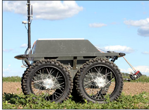
Fig. B.3: The UGV is based on a the RobuROC4 platform from Robusoft. It is a skid-steered, four-wheel driven vehicle with custom onboard computer, sensor suite, and camera setup.
