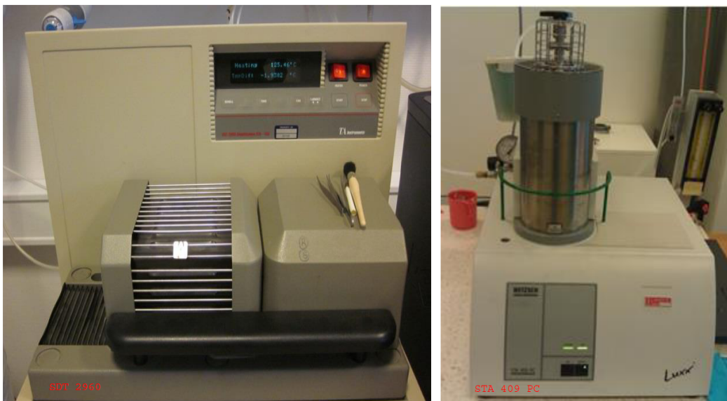
FIGURE 4.3: TGA equipment used during study
