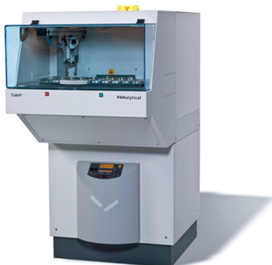
FIGURE 4.10: The PANalytical CubiX PRO X-ray diffractometer used in this study.
