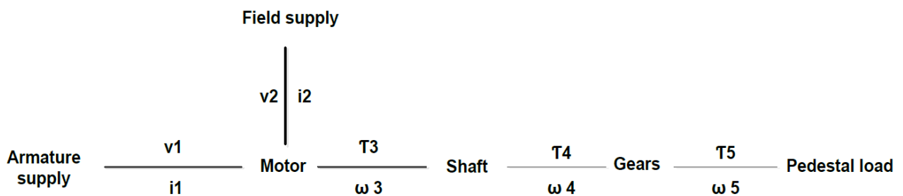
Figure 3 Word bond graph for the Antenna system.
