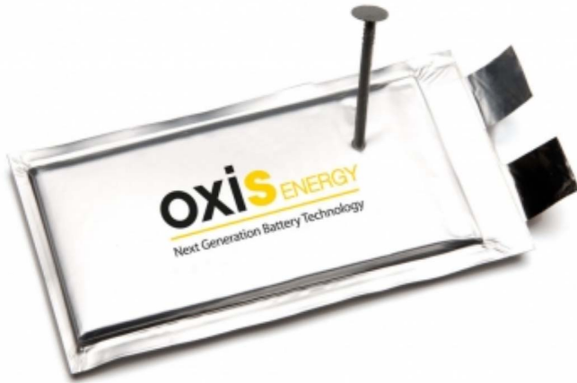
Fig. 2: Iron nail penetration of Li-S cell [5].
