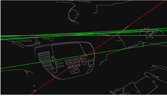
Fig. 4: Detected lines in the image. Red lines are discarded due to too much of a skew to constitute the dashboard edge.
