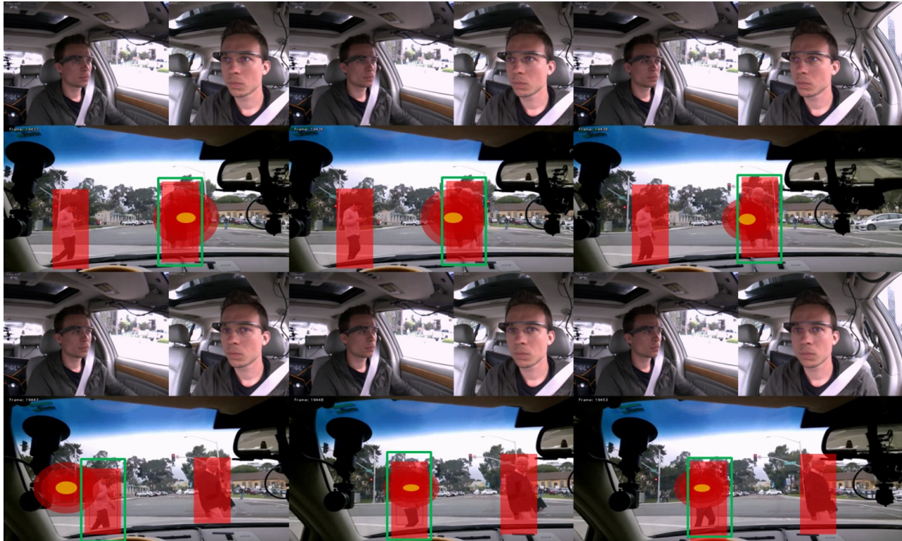
Fig. 10: Visualization of the LILO attention result in a sequence where gaze switches from one salient location to other. The red box around the pedestrian illustrates the salient region, the Gaussian kernel with yellow center shows the gaze location in the driver’s field of view. The solid box is the pedestrian that is the subject of the driver’s attention as detected by the full system.
