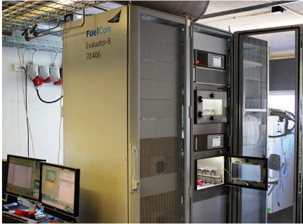
Figure B.1: FuelCon battery test station.
