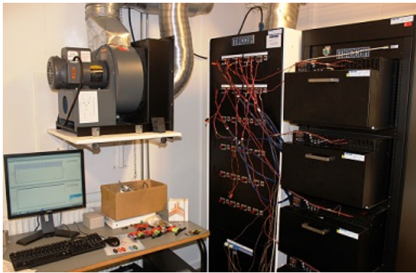
Figure B.2: Maccor battery test station.
