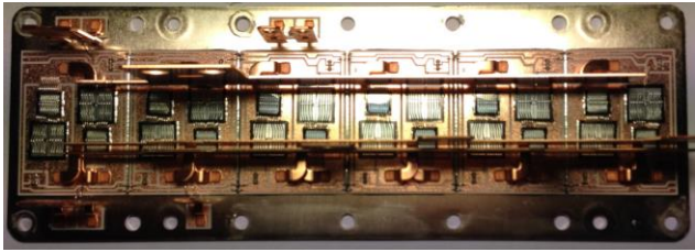
Fig. 4. Geometry of the 1.7 kV/1 kA IGBT power module with six sections in parallel.
