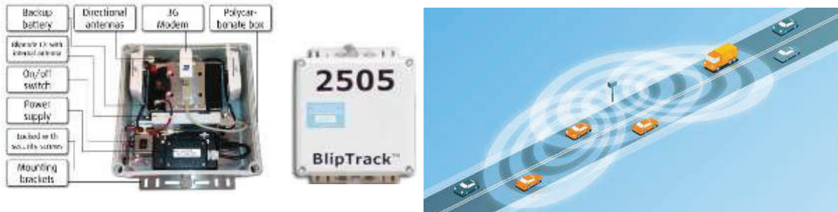
Figure 2-4. BlipTrack™ sensors and their detection zone (Source: Blip Systems)
