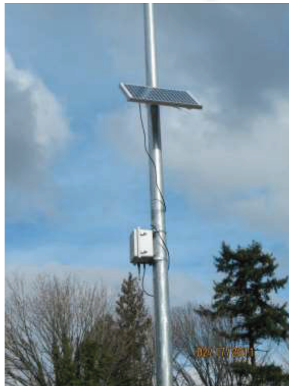
Figure III-7. BlueTOAD sensor design and components
