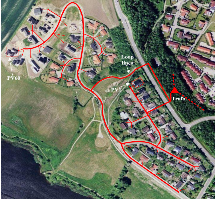
Fig. 5.2. Single transformer and its associated downstream connections of Braedstrup grid
