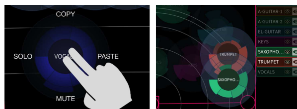
Fig. 4: Left: Touching the widget with two fingers brings up a menu providing additional settings. The user then moves up, down, right or left and releases to select the menu point. Right: Visual layers provide ability to show hide certain widgets.
