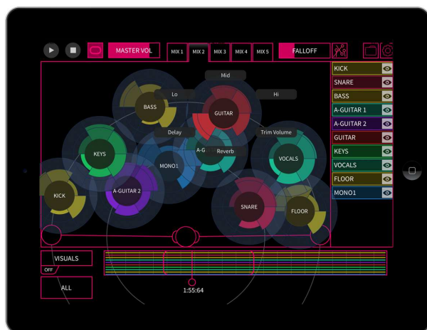
Fig. 1: Overview of the main interface. Widgets represent audio channels, which are positioned in relation to the listening position represented by the pink listener icon in the bottom centre of the stage view. The distance from the listening position determines the volume of the corresponding audio channel. The angle determines the panning.
