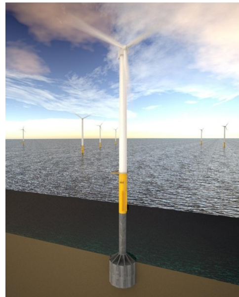
Figure 1: An illustration of a wind turbine on a bucket foundation. (Universal Foundation A/S, 2013)
