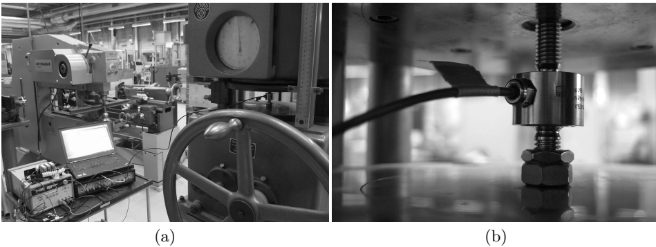
Figure B.3: (a) An overview on force transducer calibration set-up; (b) zoom to the transducer fixation in a machine
