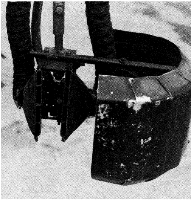
Fig. 1—Flat air nozzle unit mounted on sprayer.
