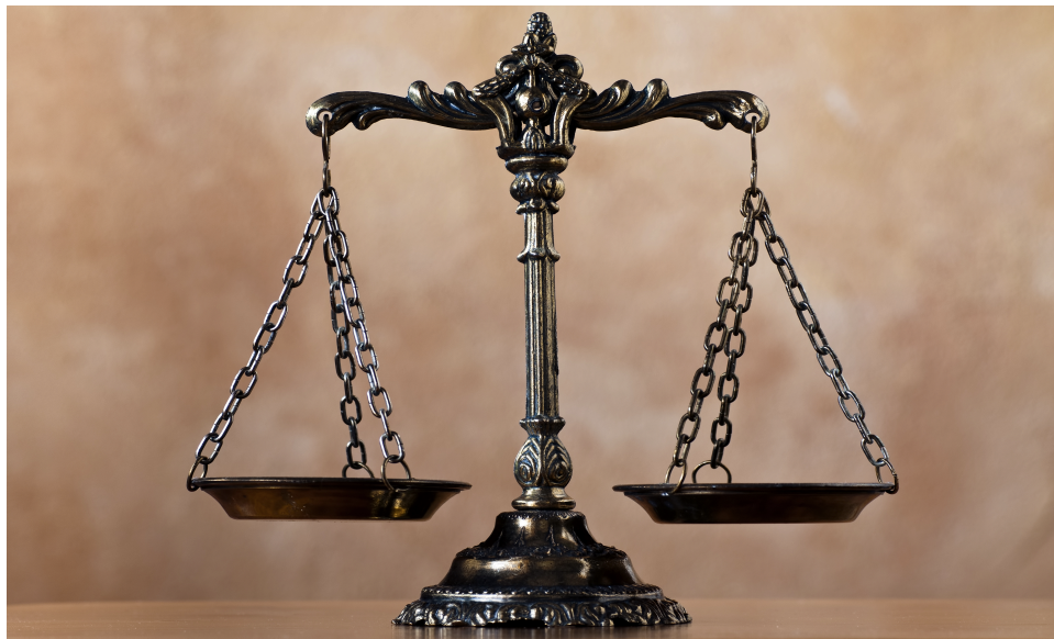
Picture 01: Within this archaic mechanism, two pans hang from a beam at points equidistant from the fulcrum (point of support). Objects were weighed by equalizing the weight with standard weights added together. At that moment, equilibrium was reached.
