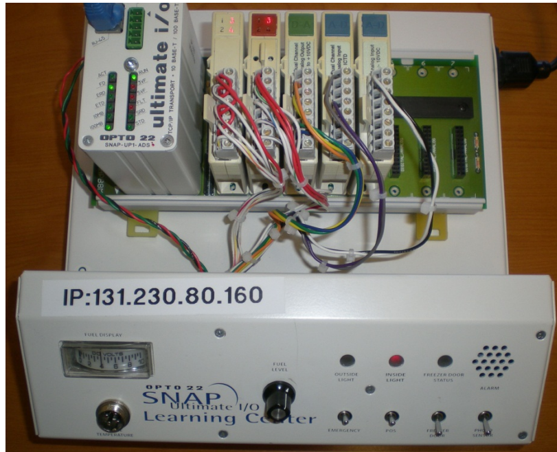
Figure 1. PAC Learning Center with PAC (upper left) mounted on rack with input/output modules. An Ethernet cable inserted in the RJ-45 jack (upper left corner) connects the PAC to a LAN.
