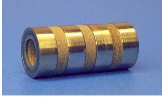
Fig. 1.20 - Tubular PbTe module consisting of four thermocouples connected with nickel bridges.
