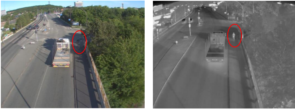
Figure 1 - Shadows complicates the detection of a cyclist in the RGB recordings, whereas the cyclist is easily distinguished from the background in the thermal recording.
