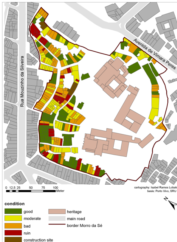
Figure 3: Condition of buildings in Morro da Sé
