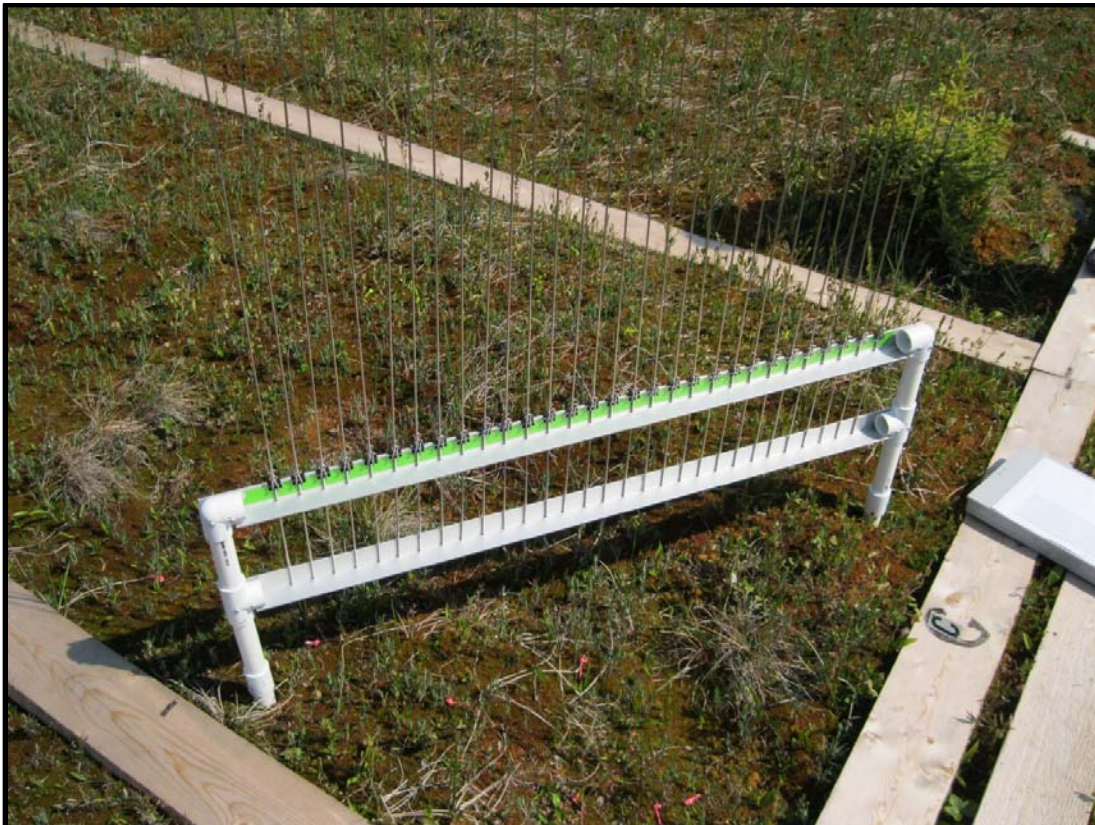
FIGURE 3.1 Point frame sampling apparatus being used in the FEN – Arm 1 – Control plot.
