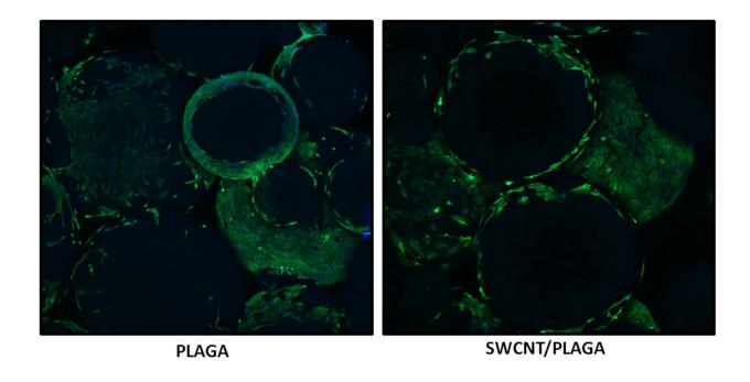
Figure 4-7: Immunofluorescence staining (green: β-actin, blue: hoechst stain) images captured using a confocal microscope (at 10X 3.1zoom). MC3T3-E1 cells adhered, grew and retained morphology on both PLAGA and SWCNT/PLAGA composites.
