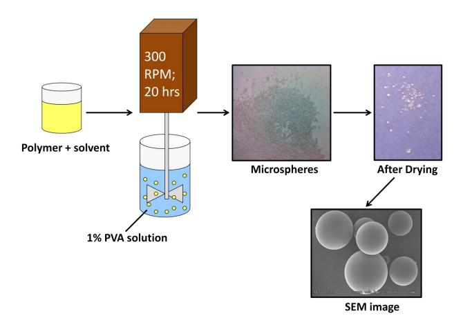
Figure 4-1: Fabrication of PLAGA microspheres using oil-in-water emulsion method. In addition, figure also shows SEM image for PLAGA microspheres demonstrating uniform shape and smooth surface.
