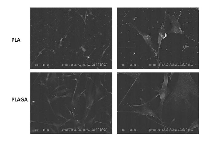
Figure 2-4: SEM micrographs of MC3T3-E1 cells cultured on PLA and PLAGA scaffolds (at 300 and 1000X magnifications). MC3T3-E1 cells adhered and grew on all the surfaces.
