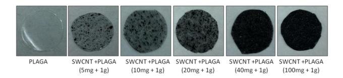
Figure 3-3: Disks (12mm diameter) cut from the PLAGA and SWCNT/PLAGA composites.
