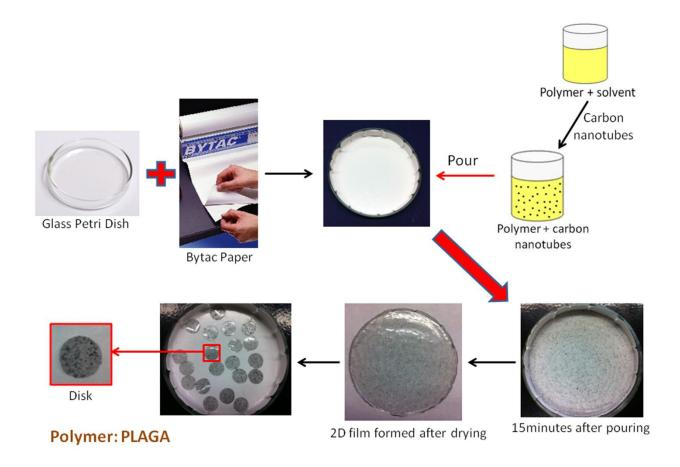
Figure 3-1: Schematic representation of steps involved in fabrication of 2-D SWCNT/PLAGA scaffolds using solvent evaporation method.
