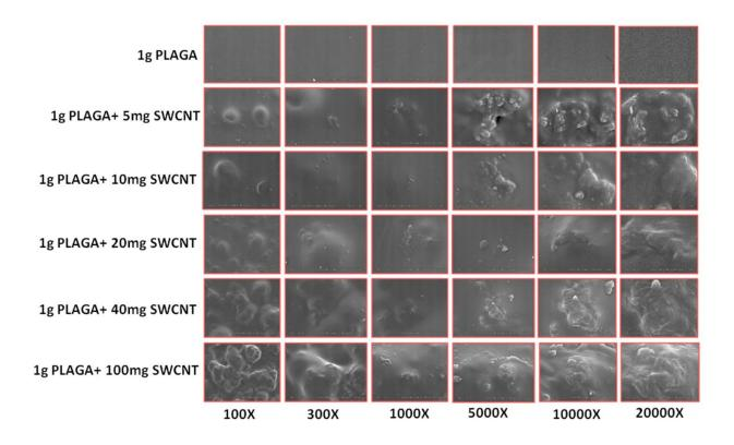
Figure 3-4: SEM micrographs of PLAGA and SWCNT/PLAGA composites (at 100, 300, 1000, 5000, 10000 and 20000X magnifications). SWCNT can be seen homogenously distributed in PLAGA matrix.
