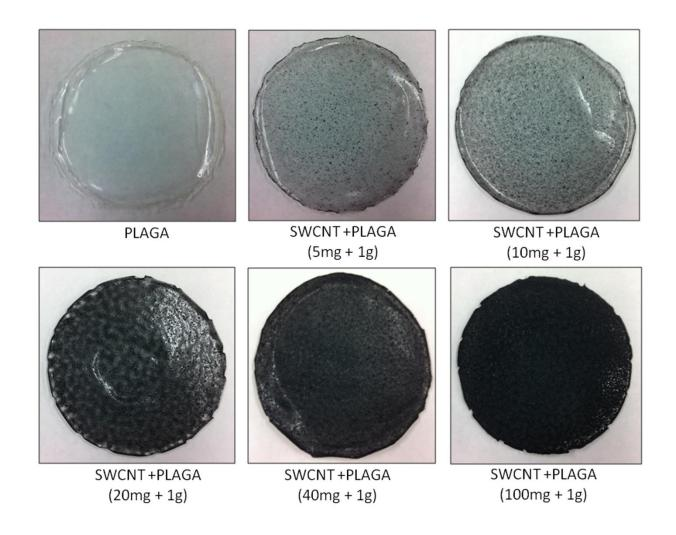
Figure 3-2: Images of 2D PLAGA and SWCNT/PLAGA composites (100mm diameter) obtained.
