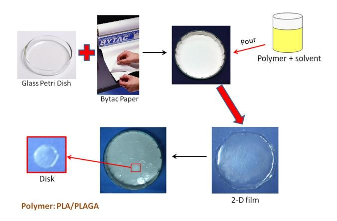
Figure 2-1: Schematic representation of steps involved in fabrication of 2-D PLA and PLAGA scaffolds using solvent evaporation method.
