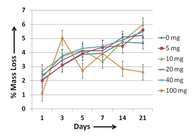
Figure 3-5: Degradation profile of PLAGA and SWCNT/PLAGA composites as a function of % mass loss over time (days). Results show no significant difference in the degradation rate of SWCNT/PLAGA composites compared to PLAGA. Data represents mean ± SEM.
