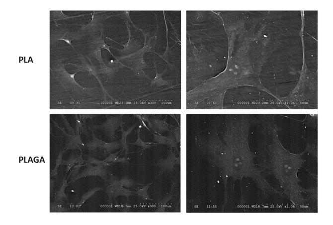
Figure 2-5: SEM micrographs of rMSCs cultured on PLA and PLAGA scaffolds (at 300 and 1000X magnifications). rMSCs cells adhered and grew on all the surfaces.
