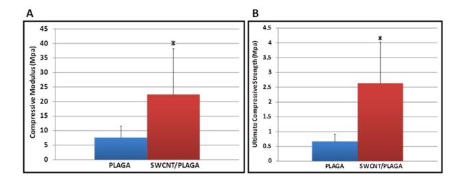
Figure 4-5: Compressive Modulus (A) and Ultimate Compressive Strength (B) of PLAGA and SWCNT/PLAGA composites. \* represents significant difference (p<0.05) compared to PLAGA.
