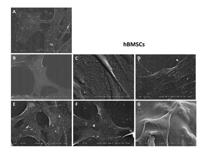
Figure 3-6: SEM images (at 1,000 X) of hBMSCs cultured on TCPS (A), PLAGA (B), and SWCNT/PLAGA composites (C–G). hBMSCs adhered and grew on all the surfaces.
