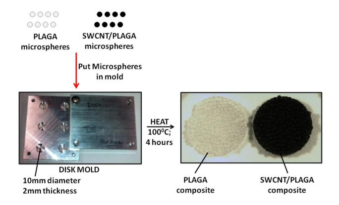
Figure 4-3: Fabrication of 3-D PLAGA and SWCNT/PLAGA composites using thermal sintering technique.
