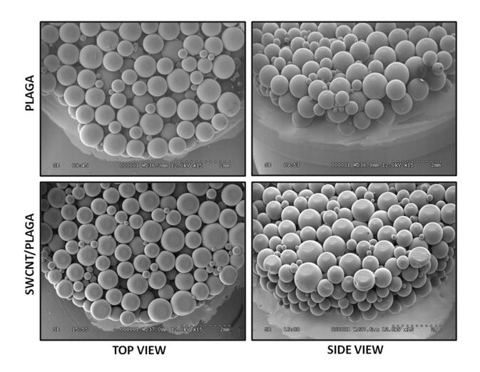
Figure 4-4: SEM micrographs of PLAGA and SWCNT/PLAGA composites. The microspheres bonded in a random packing arrangement while maintaining spacing, resembling trabeculae of cancellous bone.
