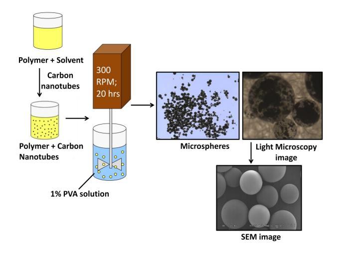
Figure 4-2: Fabrication of SWCNT/PLAGA microspheres using oil-in-water emulsion method. In addition, figure also shows light microscopy and SEM image for SWCNT/PLAGA microspheres demonstrating uniform incorporation of SWCNT into PLAGA, and uniform shape and smooth surface of the microspheres.
