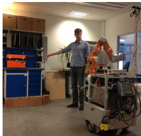
Fig. 1. The considered scenario: human is indicating an object to the robot through a pointing gesture
