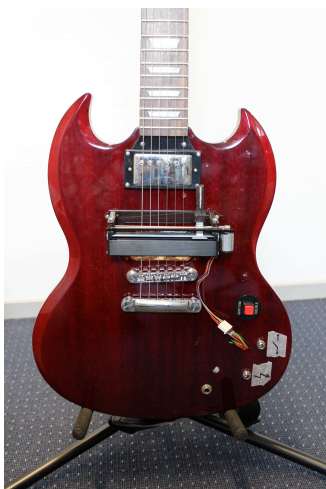
Figure 2: The Actuated Guitar. The actuator pulling the pick across the strings is a motorised fader from a mixing console. The motor is controlled via a Arduino microcontroller and a 2Motor motor controller mounted inside the guitar's body.
