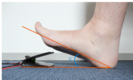
Figure 3: The pedal used for strumming the guitar. The height of the pedal will increase or decrease the angle X and thereby alter the difficulty and the intensity of the exercise.
