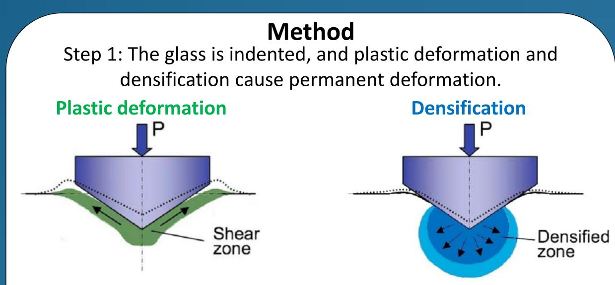
Step 2: The indent is mapped by AFM before and after annealing at  $0.9 \times T_g$  for 2 hours. The annealing fully recovers the densified volume.
