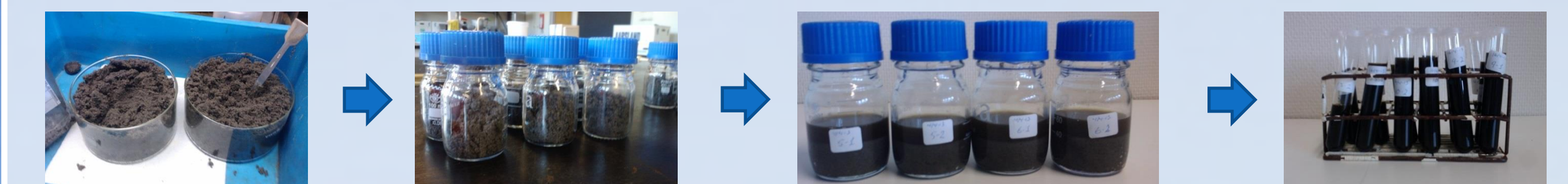
Fig. 3: The contaminated soil/ surfactant water ratio used in this test was 4 g/mL. No extra DNAPL was added.
