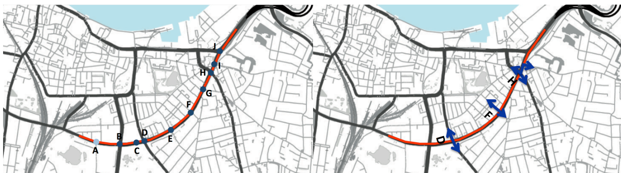
Figure 3. The studied section and the included intersections covered with ATCS (left) and the crossing bus routes (right) on the ring road.
