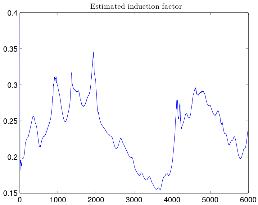
Figure 5.8: Induction factor estimate for full-scale test at mean wind close to rated.
