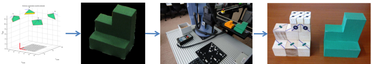
Figure 1: The major steps of the procedure from left to right: Image acquisition by the four-camera system, background subtraction, assembly planning using a robotic system, final object assembled by wooden cubes.
