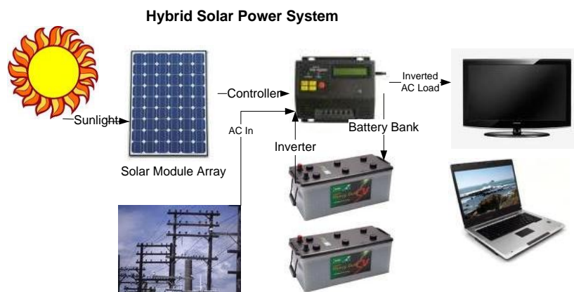
Figure 3. Hybrid Solar Power System for SCR power backup
