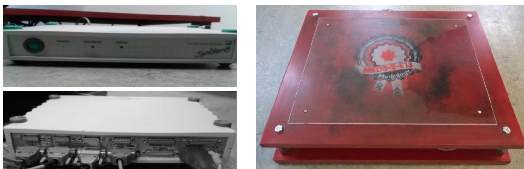
Spider 8 data logger (left) and balance board (right).
