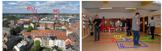
Fig. 1. Left: View from BS2 towards measurement location. Right: Users during measurements, with the user squares and orientations A–D indicated.
