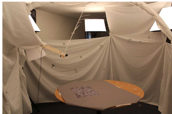
Figure 3: Top: An image of the setup. The test subjects are only able to watch the monitor and not the scene. Furthermore, they are able to rotate the metal arm on which the monitor is attached. Bottom: An image of the scene that the web-camera captures. Using a protruding stick the web-camera was positioned closer to the centre to be able to track the marker and to be able to see details in the objects.
