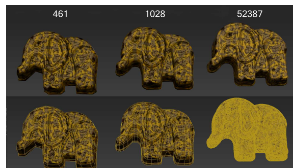
Figure 4: From left to right: The specular toy elephant in two low complexity versions, as well as the scanned original. Bottom row shows the same objects in wire frame. The polygon count is noted in the top.
