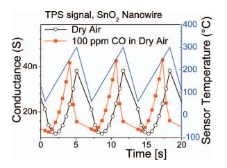
FIG. 3. (Color) Temperature-programed sensing (TPS) measurements, where the blue triangular wave (top) is the temperature profile of the sensor in time, and the black circles and red squares show the nanowire conductance measurements upon exposure to dry air and 100 ppm CO, respectively. The distinct differences between the signal patterns can serve as a means of discrimination.
