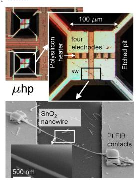
FIG. 1. (Color online) Top: optical image of a typical  $\mu$ hp architecture. Bottom: SEM image of the individual SnO<sub>2</sub> nanowire integrated as a chemiresistor using FIB technology.
