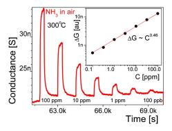
FIG. 4. (Color online) Conductance response to NH $_3$  pulses in air (100 ppm-100 nmol/mol (ppb) step  $\sqrt{10/10}$  power law) measured at 300 °C. In the inset, the conductance increase as a function of NH $_3$  concentration is shown (log-log scale). The solid line shows the data fit with a power law curve.
