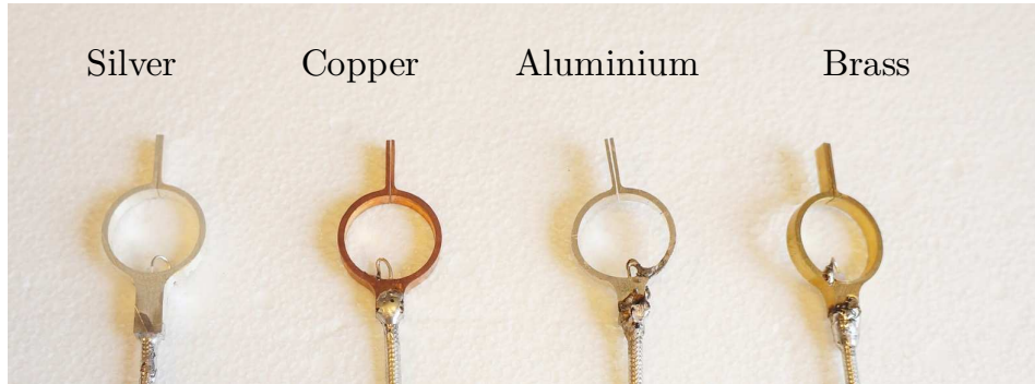
Fig. D.23: Loop antenna mock-ups with air capacitors.
