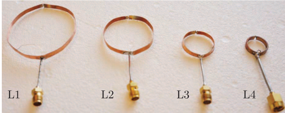
Fig. D.12: Loop antennas of four different sizes.
