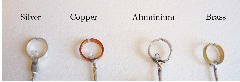
Fig. D.18: Loop antenna mock-ups with fixed capacitors.
