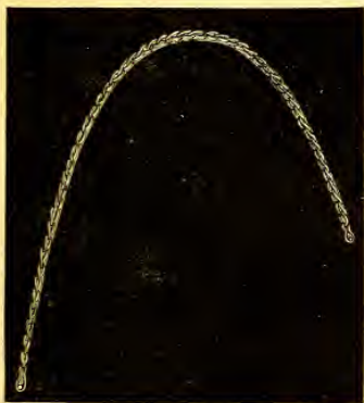
THE CATENARY, OR CURVE FORMED BY A HANGING CHAIN.
