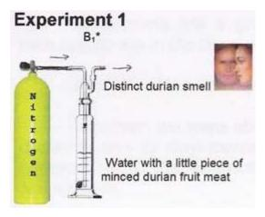
The non-reactive and odorless  $N_2$  gas is bubbled through the water containing a small piece of durian and this will carry its smell outside the bottle  $B_1$ .
