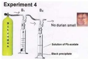
When the durian smell was passed through a solution of Pb-acetate, a black precipitate can be seen at the bottom of bottle 4.
