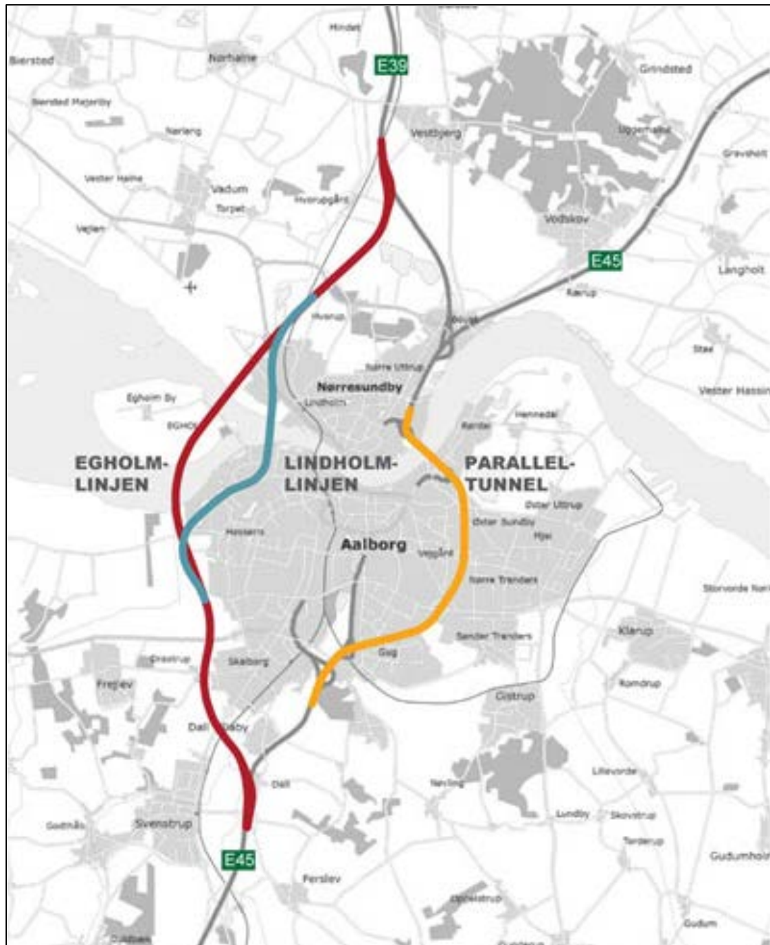
Figure 6.1: The three alternative solutions for a Third Limfjord Crossing included in the EIAs in 2003 and 2006. (Danish Road Directorate 2010)
