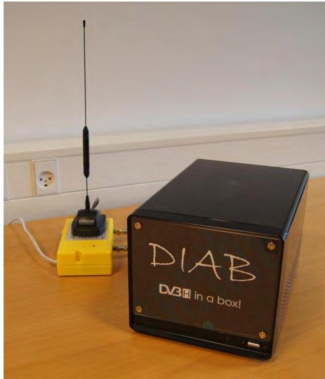
Figure 6.6: Elements of the DIAB transportable DVB-H testbed.
