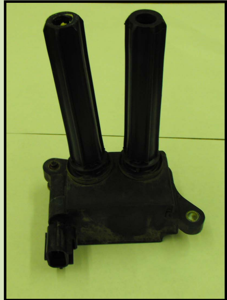
2 styles of coils that fire 2 plugs "Hemi" V-8
