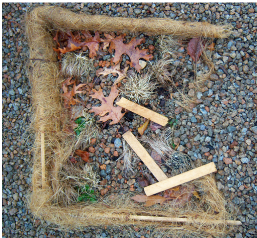
Figure 4. Coconut fiber trays are degrading at the surface of the substrate (picture by author).
