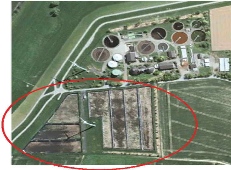
Figure 2. Reed bed facility located in Kalkar-Hönnepel, Germany. It is consisting 7 reed beds covering 20,400 m 2 (outlined in red).
