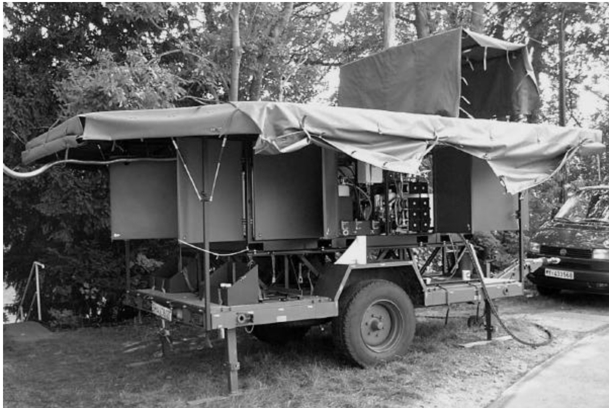
Figure 1: Photography of the mobile drinking water purification unit Kärcher TWC 1600 GT at the field site near the Teltowkanal in September 2000.
