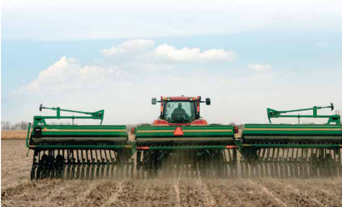
Figure 5: Great Plains 3S-3000, Thirty-foot, Three-Section Folding Drill
